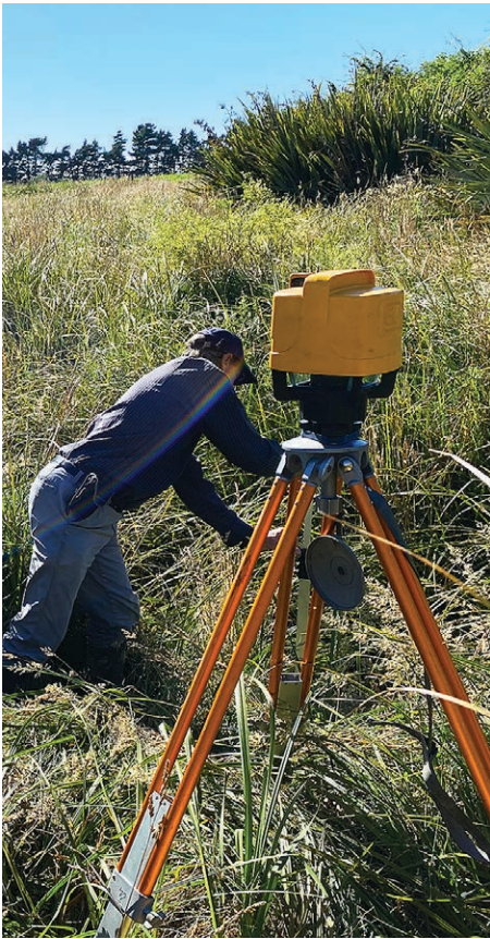
Laser levelling a potential wetland for development in the Waimea catchment as part of the Jobs for Nature funded catchment projects.
