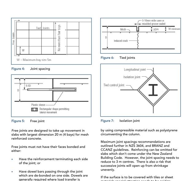
If the surface is to be covered with tiles or sheet materials special attention needs to be paid to ensure that the joints coincide with joints in the floor covering.
