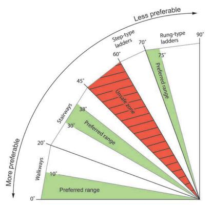
Figure 6.3 Selection of Access – Limits of Slope Angle (Adapted from AS 1657–2013 Fig 2.1)
