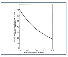
Figure 1: Approximate compressive strength of concrete made with various water/cement ratios
