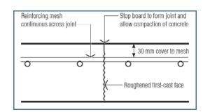
Figure 8: Construction joint
