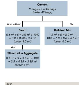
For proprietary pre-bagged concrete, the bag and instructions will indicate the approximate yield per bag. Allow for at least one extra bag in case a bag is damaged. Use the same product for the whole job.
