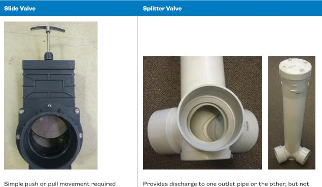
Simple push or pull movement required<br/>to open or close the valve. However, the<br/>handle needs to be enclosed in a protective<br/>chamber to avoid jamming up fromProvides discharge to one outlet pipe or the other, but not<br/>both at same time. This provides some confidence in avoiding<br/>inadvertent FDE discharge to stormwater
