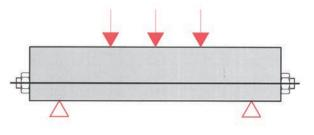
POST TENSIONED CONCRETE BEFORE LOADING
