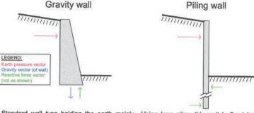
Standard wall type holding the earth mainly through its own weight. Will topple relatively easily, as the internal leverage of the earth pressure is very high. Using long piles, this wall is fixed by soil on both sides of its lower length. If the piles themselves can resist the bending forces, this wall can take high loads.
