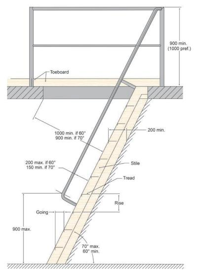
Figure 6.4 Typical Dimensions for Step-type Ladders (Adapted from AS 1657–2013 Fig 7.4)
